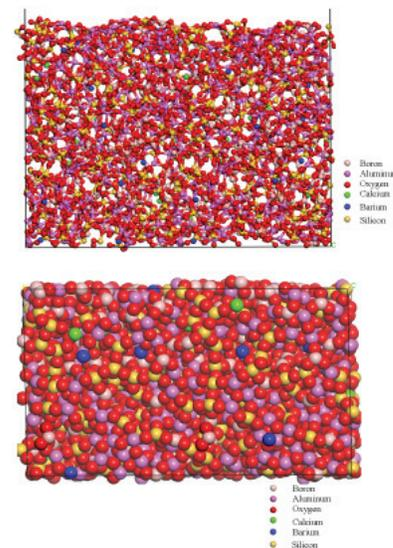
Figure 3 – A view of the AEBS glass surface a) parallel to the C-axis and b) normal to the A and B axis plane
