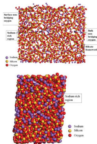
Figure 2 – A view of the sodalime glass surface: (a) parallel to the C-axis and (b) normal to the A and B axis plane
